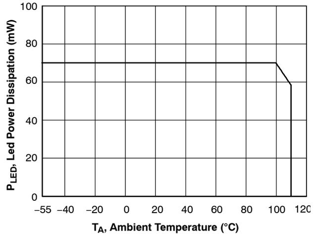
Figure 14. Led Power Dissipation vs. Ambient Temperature (FOD817)
