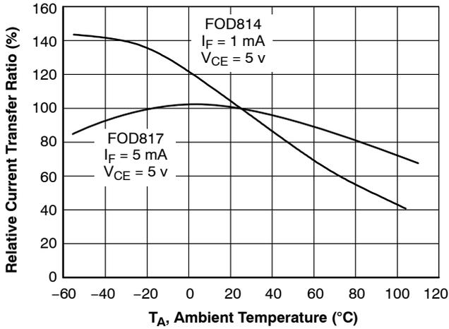
Figure 11. Relative Current Transfer Ratio vs. Ambient Temperature
