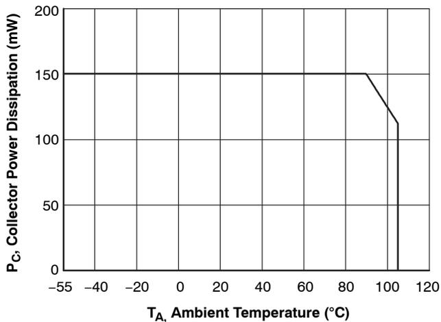
**Figure 3. Collector Power Dissipation vs. Ambient Temperature (FOD814)**
