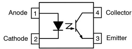
Figure 2. Schematic – FOD817
