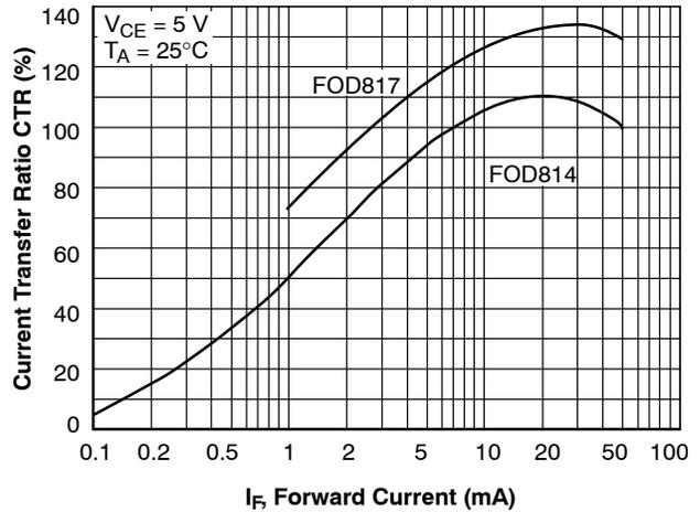
**Figure 8. Current Transfer Ratio vs. Forward Current**
