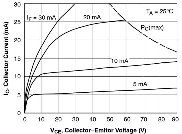
**Figure 10. Collector Current vs. Collector-Emitter Voltage (FOD817)**
