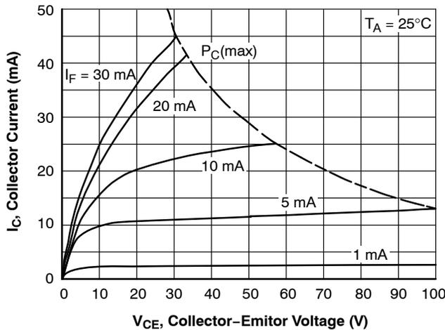
**Figure 9. Collector Current vs. Collector-Emitter Voltage (FOD814)**
