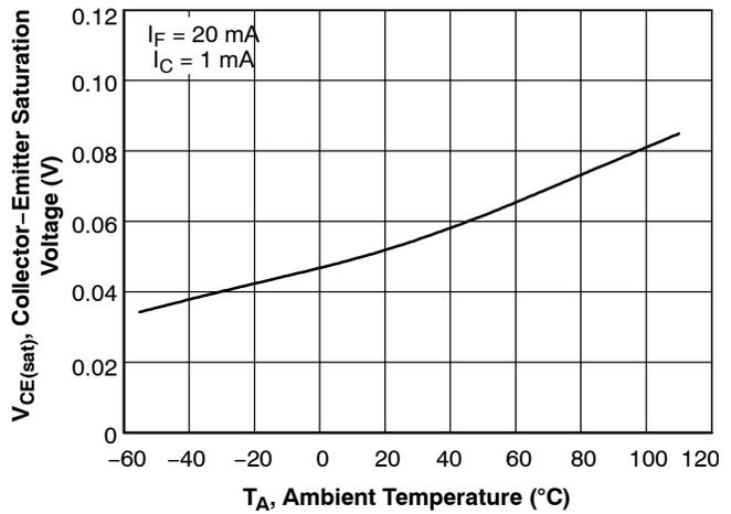
Figure 12. Collector-Emitter Saturation Voltage vs. Ambient Temperature
