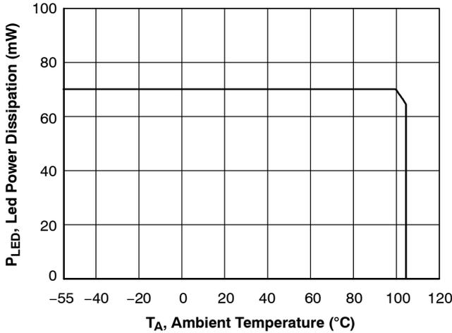
Figure 13. Led Power Dissipation vs. Ambient Temperature (FOD814)
