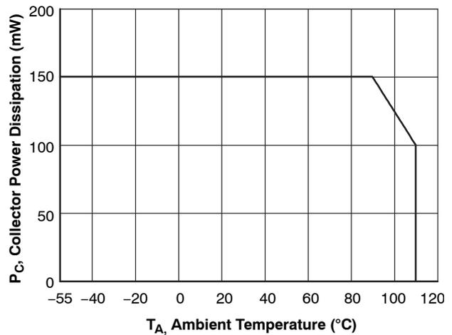
**Figure 4. Collector Power Dissipation vs. Ambient Temperature (FOD817)**
