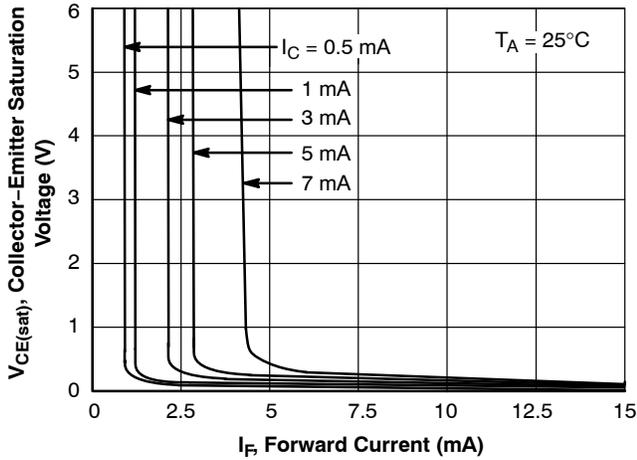
**Figure 5. Collector-Emitter Saturation Voltage vs. Forward Current**
