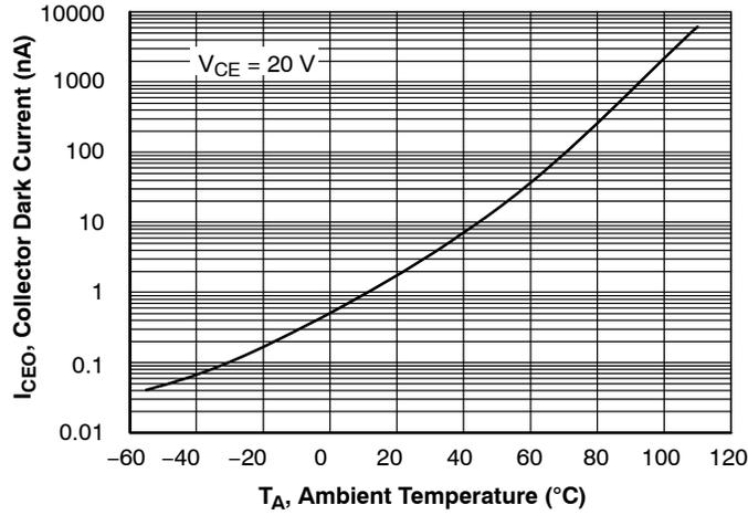
Figure 17. Collector Dark Current vs. Ambient Temperature
