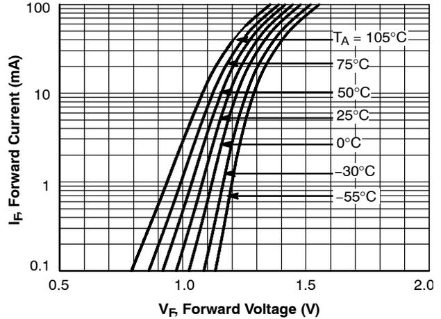
**Figure 6. Forward Current vs. Forward Voltage (FOD814)**
