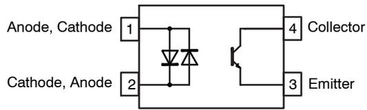
Figure 1. Schematic – FOD814
