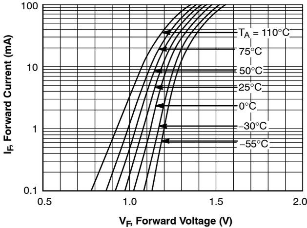
**Figure 7. Forward Current vs. Forward Voltage (FOD817)**
